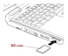
Figure 8-5 Inserting an SD card
